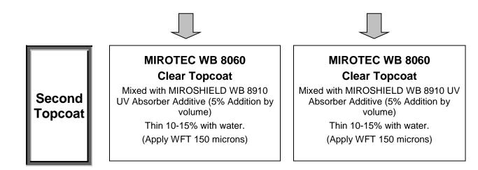
MIROSHIELD SB 3900 & WB 8910 UV Absorber Additives increase the durability of the clear coating to which they are added.
